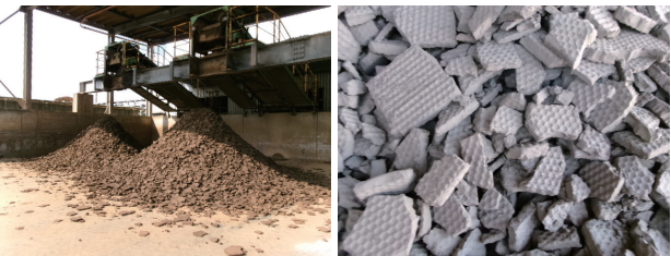
Drying sludge to make press cake.
